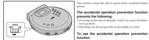
This function causes the unit to ignore short, accidental button "**O**—" When the unit is in the hold mode according to the HOLD
